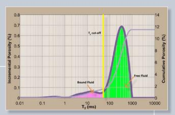
Figure 1 - T, distribution showing integral for free fluid
