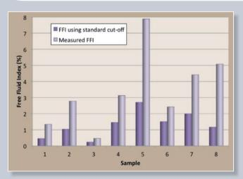
Figure 3 – Free Fluid Index using standard and measured cut-off values
